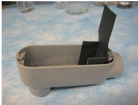
Figure 1-2: Place the folded cardstock box into the conduit body. The long-side portion of the cardstock box faces upward and will be used to conceal the webcam from other light sources when in use.
