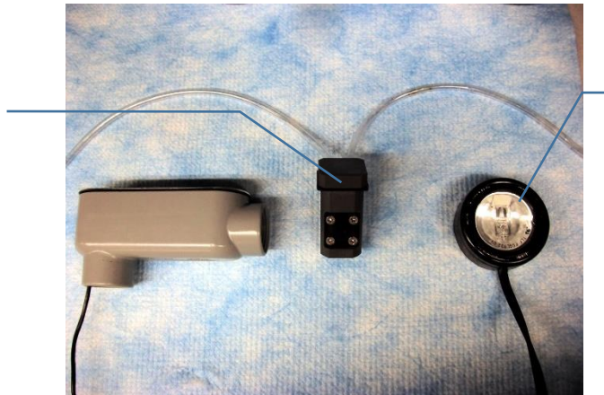
Figure 5-1: Example setup for the determination of nitrate concentration in drinking water with a flow-thru sample cell and a xenon light source. No actual data has been acquired at this time.
