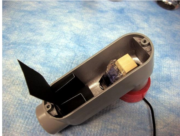
Figure 4-1: Firmly place the webcam and wooden wedge in the center of the conduit body.
